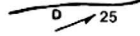
Reverse fault, showing bearing and plunge of relative movement of downthrown block (D)
